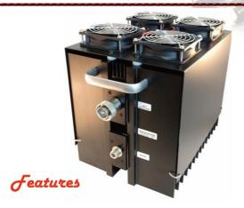
Type N or DIN 7/16 stainless steel M/F connectors per MIL-STD-348A, interface dimensions mate nondestructively with MIL-PRF-39012. Designed to meet MIL-DTL-3933 environmental specification. DIN 7/16 connector, conforms to DIN 47223, IEC 169-4, VG 95250, CECC 22190. Forced air cooling.
