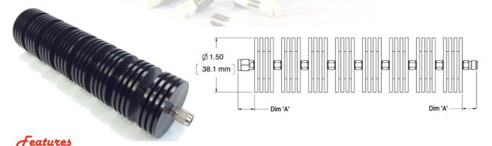
Precision 2.92 mm stainless steel M/F connectors per MIL-STD-348A, interface dimensions mate nondestructively with MIL-PRF-39012. Designed to meet MIL-DTL-3933 environmental specification. Compact construction meets a wide range of design requirements.
